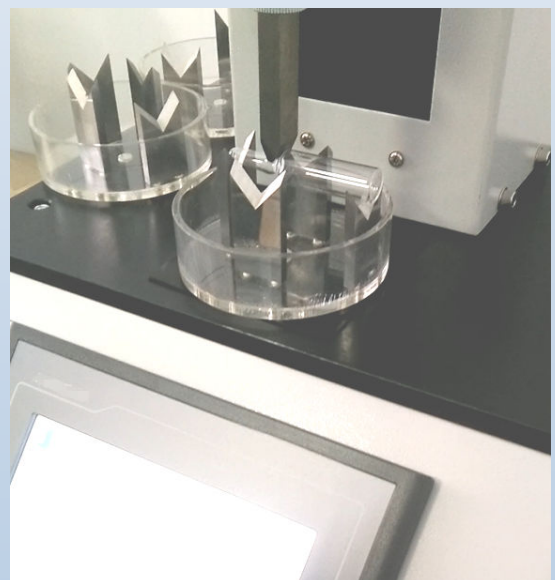
Test set-up for determining the force for breaking ampoules
